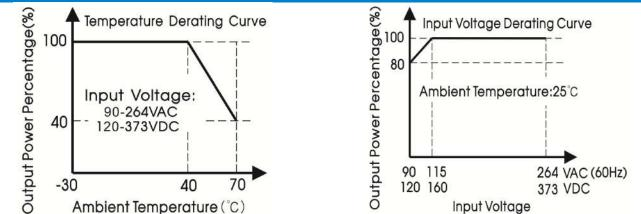
Note: 1) With an input voltage between 90-115VAC and a DC input between 120-160VDC the output power must be derated as per the temperature derating curves;
