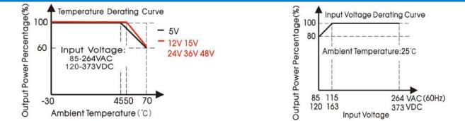
Note: 120-163VDC the output power must be derated as per the temperature derating curves;
