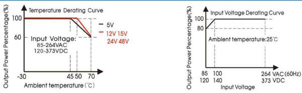
Note: ①Input voltage reduction is required on the basis of temperature reduction for the input voltage is 85 - 100VAC/120 - 140VDC; ②This product is suitable for applications using natural air cooling; for applications in closed environment please consult factory or one of our FAE.
